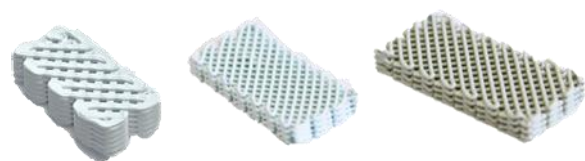
Sintered (two left) and green (right) samples, printed with Filament-Oss 50HA
