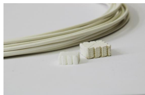
Sintered (Left) and green (right) samples, printed with FILAMENT-Cer ZrO 2
